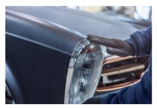
thoroughly overhauled, the interior is elaborately restored, the body is given a cataphoretic dip primer coat as can be found on modern production vehicles and then undergoes a comprehensive rust protection treatment before receiving its final paint finish.
